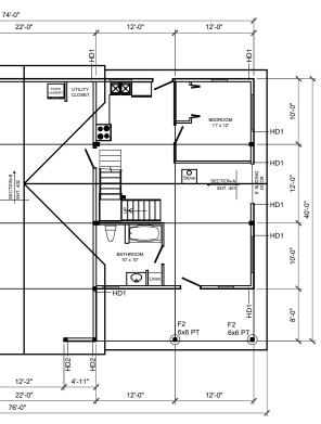
NOTES: HD1 - SIMPSON HDU8 w/ SSTB24 ANCHOR BOLT (MAY REQUIRE DEEPENING FTG. IN A.B. REGION) HD2 - SIMPSON HDU11 w/ SSTB28 ANCHOR BOLT
