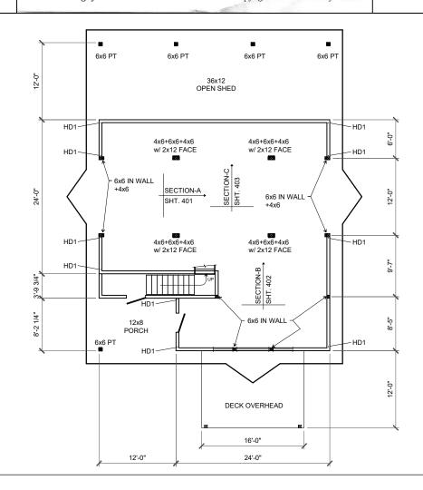
HD1 = SIMPSON HDU11 w/ SSTB16 ANCHOR BOLT
